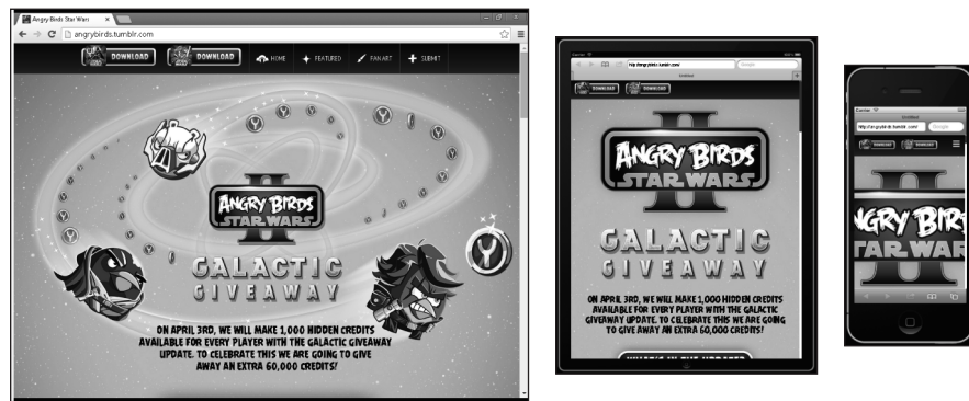
FIGURE 1-2: The Angry Birds Star Wars page optimized for desktop, tablet, and mobile using Bootstrap.
