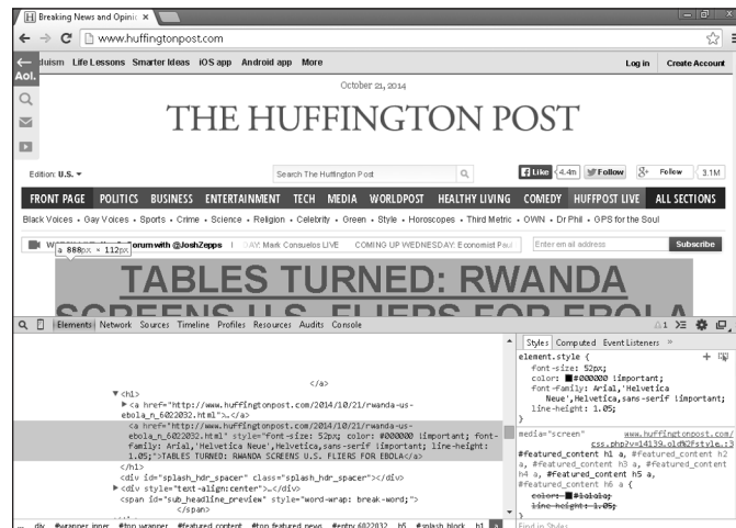
FIGURE 2-2: The blue highlighted code is used to create the web page headline.
