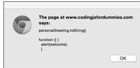
FIGURE 3-3: A closure includes the code of the returned inner function.
