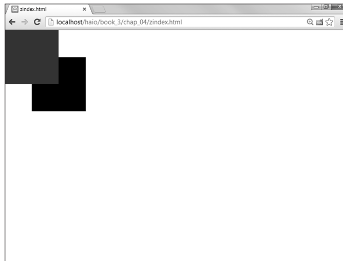
FIGURE 6-3: The z-index allows you to change which elements appear closer to the user.
