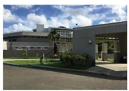
The Editorial Universitaria building is a three-story, site cast structure. The building, constructed in approximately in 1997 and is reinforced concrete walls and roof, on a 6" reinforced concrete slab on grade with interior and exterior grade beams. The roofing system is a BUR and corrugated metal. The interior finish generally consists of painted concrete and drywall walls, VCT, vinyl laminate, and ceramic tile. The 3rd floor is covered corridor covered with tinted, laminated, Plexiglas.
